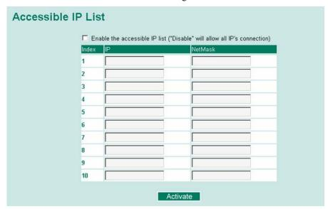
You may add or remove IP addresses to limit access to the PT-7728. When the accessible IP list is enabled, only addresses on the list will be allowed access to the PT-7728. Each IP address and netmask entry can be tailored for different situations:
